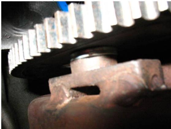
bottom out in the trans pump again causing early failure. When unbolted and pushed back into the trans, there should be around 1/8<sup>th</sup> inch air gap between the flywheel and the converter mount pads on a 4L60E. If it is not, you shim it to get the proper distance. I had a little trouble with this next part. The material you use is grade 8 washers. Wait, what? The fate of the entire drivetrain is bound with bolts and
