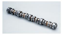
lumpy stick. Yes, get over it cowboy that fancy LS3 is controlled by a lumpy stick...still, cause it works. The lumps or lobes are cast to open the correct valve at the correct time via a lifter and push rod. Going to be tough, but picture in your melon an egg shaped lobe on the cam. As it turns the
